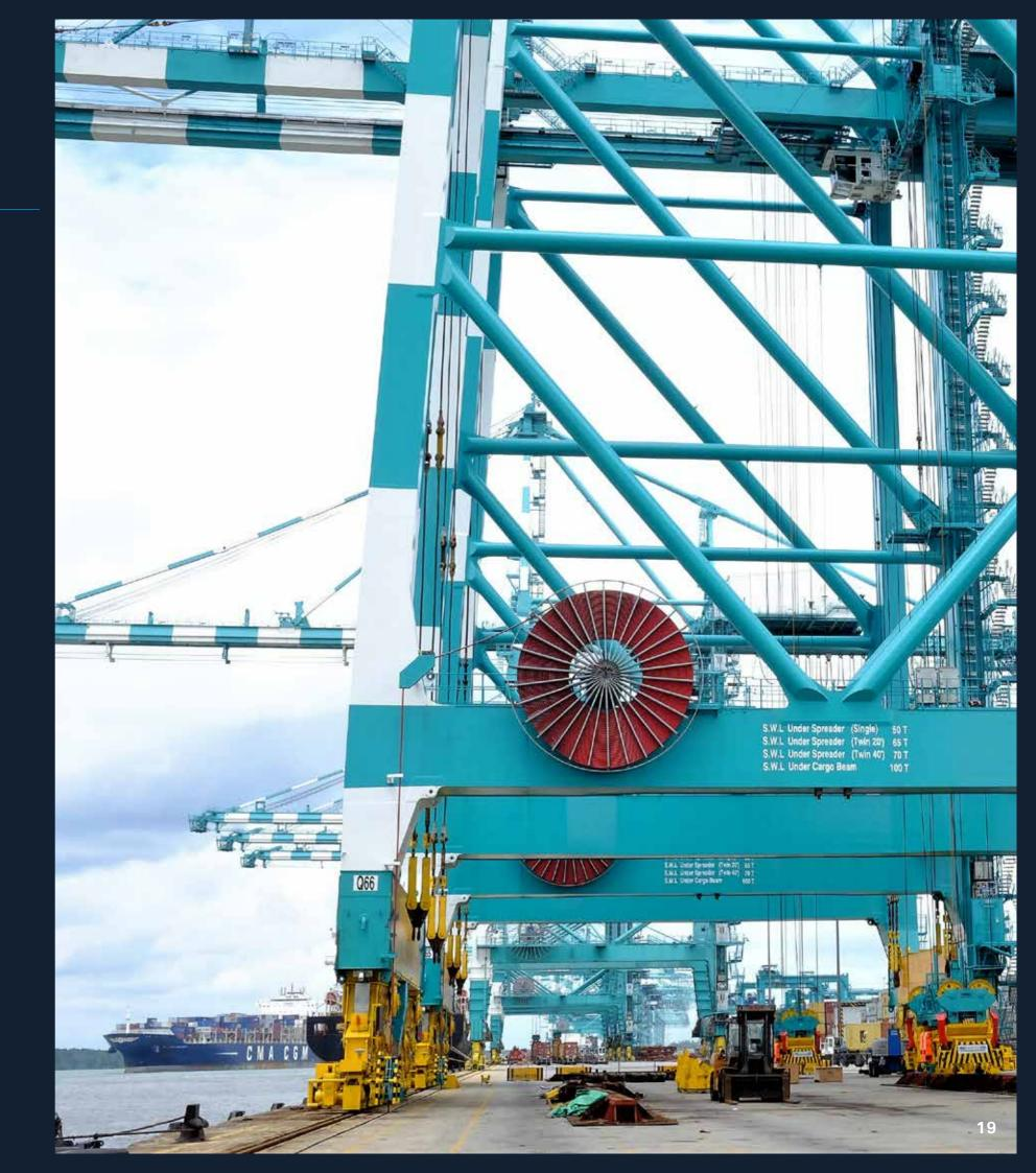
Cavotec's extensive experience and comprehensive range of innovative technologies help customers to connect and electrify STS, RTG, ASC, RMG and mobile harbour cranes, thereby improving efficiency and reducing environmental impact.
