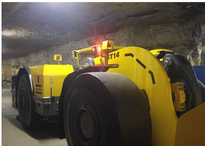
ST14 underground loader equipped with cameras and Media Base Unit
