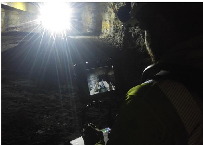
Operator maneuvering the ST14 underground loader with the Radio Remote Control mounted with tablet
